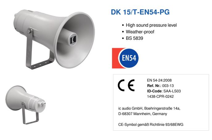
The 15W powered speaker is equipped with a 100V line transformer with 4 power adjustments, also lowimpedance operation (20 ohms) is possible. The impact-resistant ABS housing UL94V0 in RAL 7035 guarantees long-term stability. For additional reliability, a ceramic block and a thermal fuse are provided.
