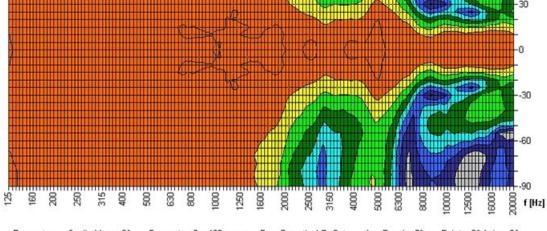
Parameters: Cyclic Move: 0° ; Symmetry: 0..+180 sym ; Freq.Smooth: 1/3 Oct ; Ang.Resol.: 5° ; Rel. to: 0° Axis 0°
